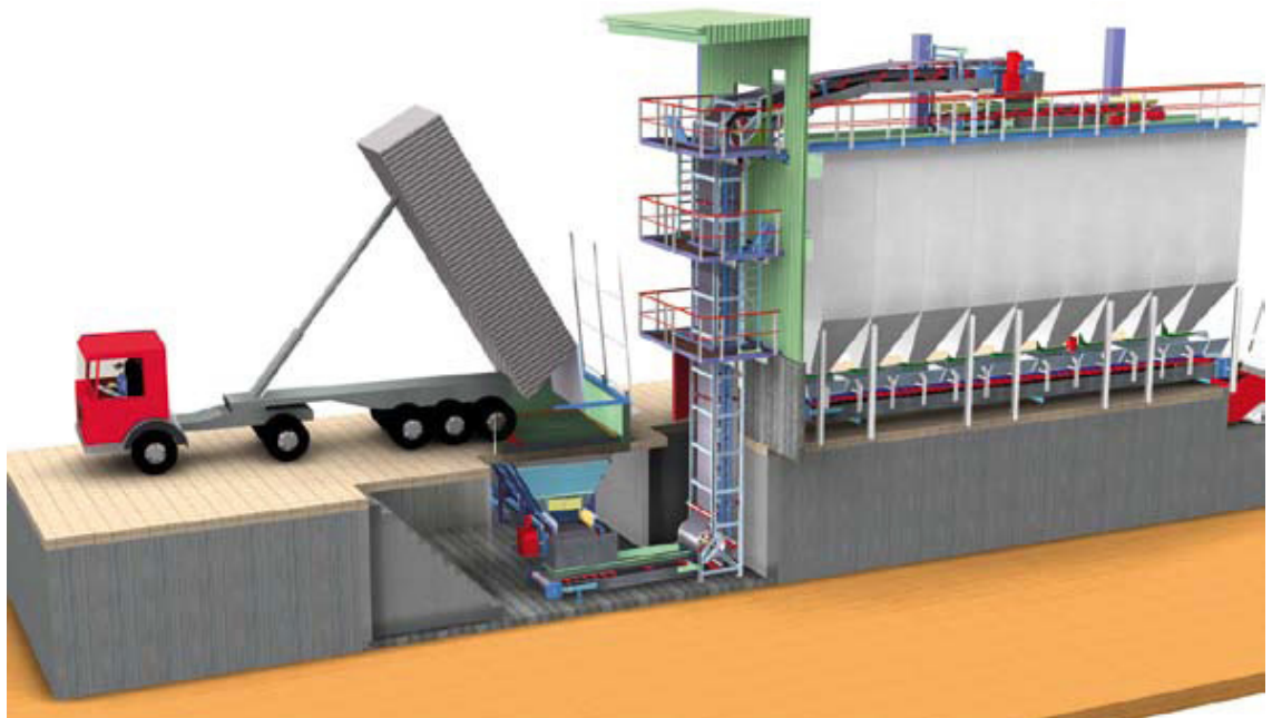
Fig. 1 Gilne GmbH: accessible discharge bunker, double belt conveyor, silo arrangement, weighing conveyor, and Kniele Cone Mixer.
