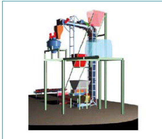
Fig. 3 Ebema: C shape conveying in double belt conveyor on cone mixer.
