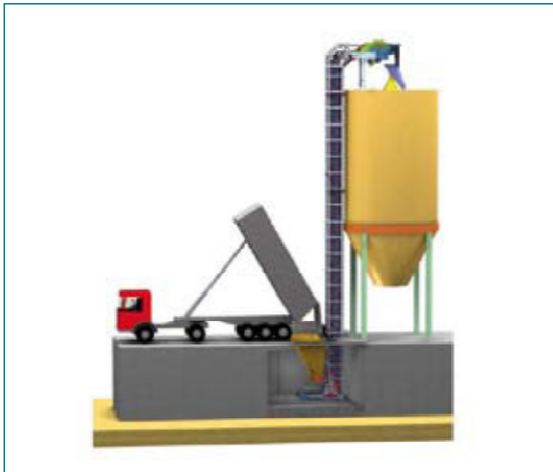
Fig. 2 TCR: bucket conveyor system replaced by double belt conveyor, rotary distributor, multi-chamber silo
