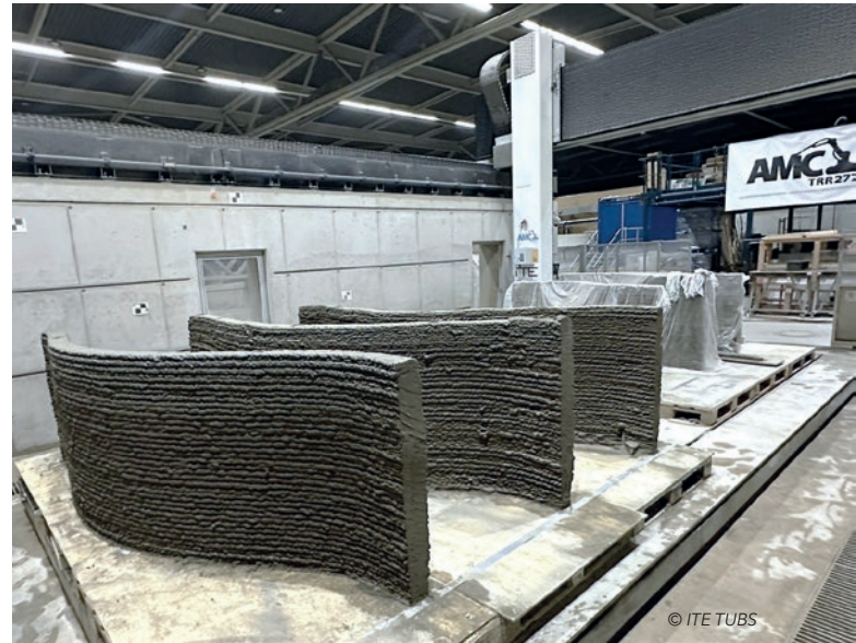
The Shotcrete 3D printing process allows for great freedom in the geometry of precast concrete elements. Single- and double-curved reinforced components can be produced in the DBFL without formwork.
