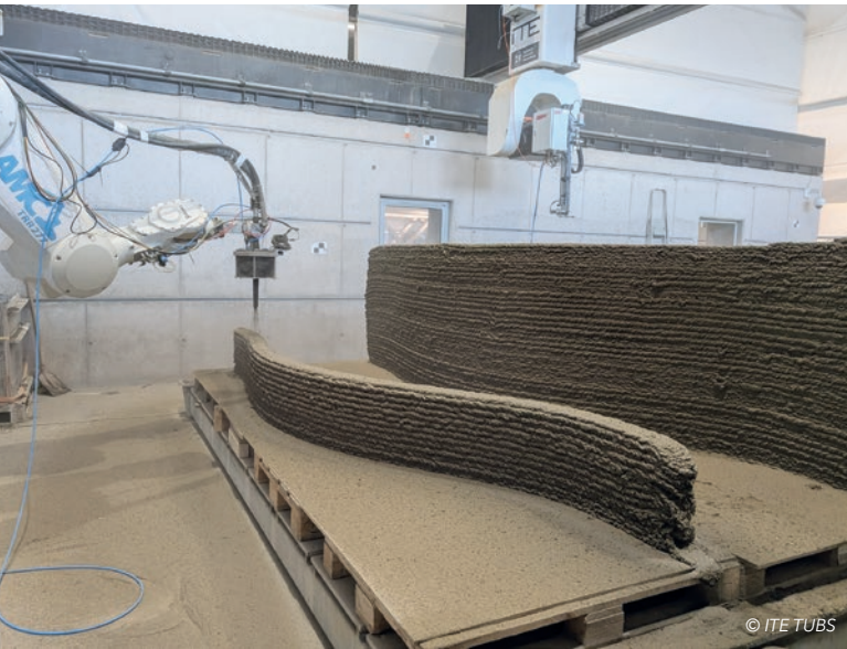
The Shotcrete 3D printing process allows for great freedom in the geometry of precast concrete elements. Single- and double-curved reinforced components can be produced in the DBFL without formwork.
