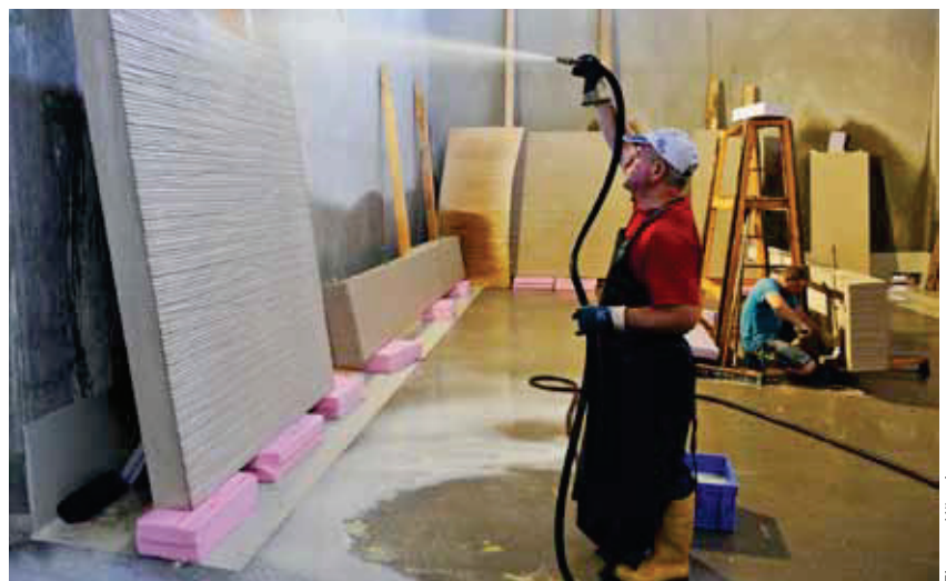
Over the last few years, a separate acid-treatment and finishing area used for the architectural concrete façades has been added
