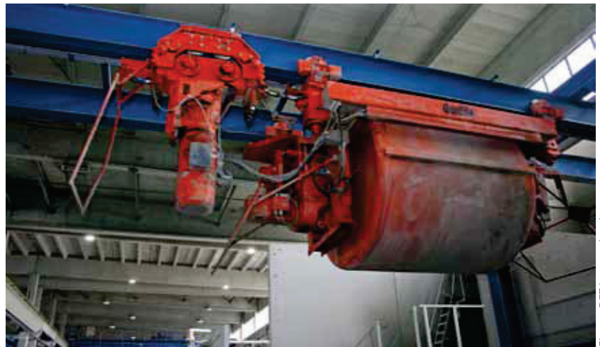
The annually produced quantity of up to 10,000 m³ of concrete is distributed to the points of placement within the production hall by a Dudik bucket conveyor
