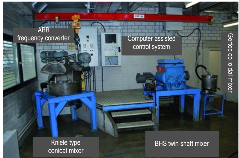
Fig. 1: Mixing plant at the Institute of Structural Concrete, TU Darmstadt
