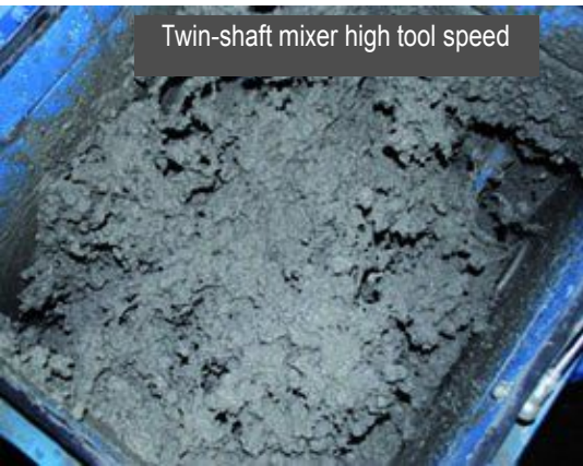
Fig. 3: Twin-shaft mixer with a high tool speed
