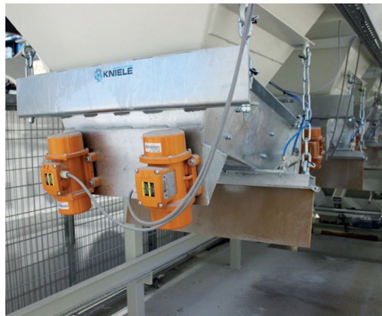
For the storage and weighing of the aggregates, Kniele has installed an in-line silo with 3 chambers (3 m 3 each) with vibrating channels for coarse and fine dosing (frequency converter-controlled).
