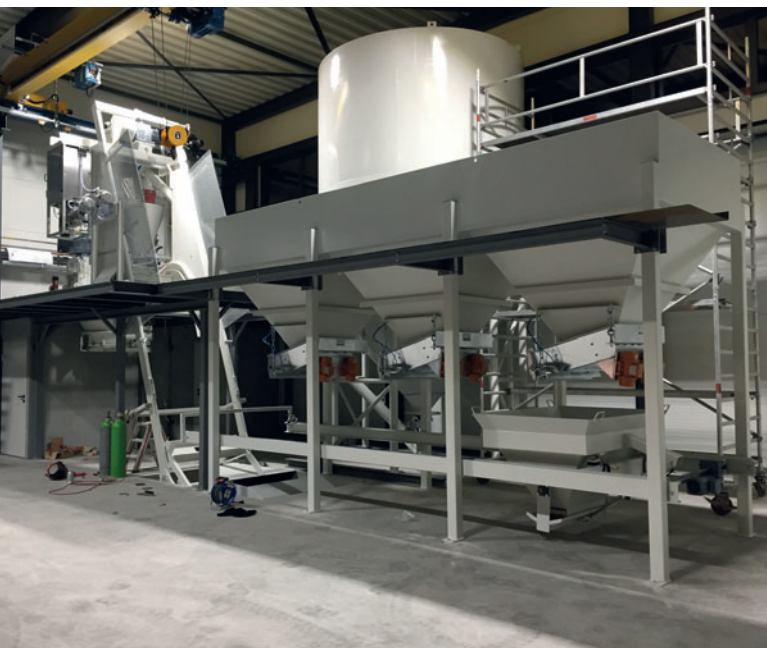
For the storage and weighing of the aggregates, Kniele has installed an in-line silo with 3 chambers (3 m 3 each) with vibrating channels for coarse and fine dosing (frequency converter-controlled).
